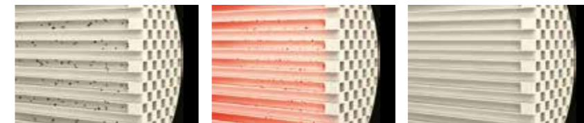
1. Particulate matter trapped 2. Regeneration starts 3. Regeneration completes*
