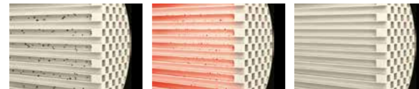
1. Particulate matter trapped 2. Regeneration starts 3. Regeneration completes*
